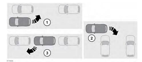
Park assist is an aid to manoeuvring the vehicle in and out of parking spaces and parking bays. Park assist takes control of the vehicle's steering system to manoeuvre the vehicle.
