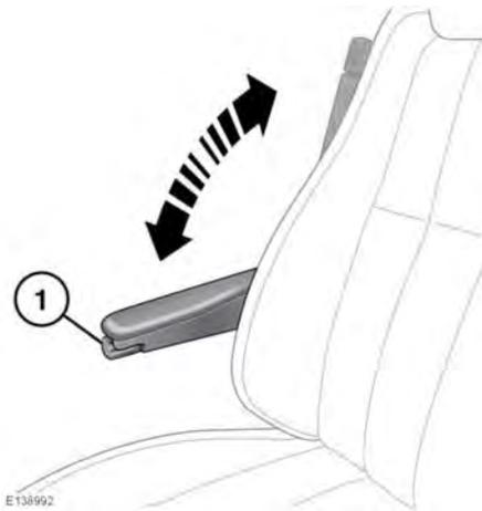
Use the adjuster wheel (1) to set the required height. The folding armrest may be stowed by moving to the vertical position.
