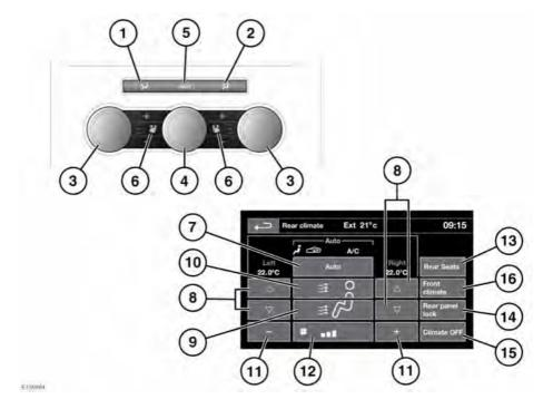
There are two types of Rear climate control: 3 Zone and 4 Zone. All of the 3 Zone controls will affect the whole of the rear passenger compartment. 4 Zone allows independent control of each side. To access the Rear climate Touch screen menu, select **Rear climate** from the **Front climate** menu.
