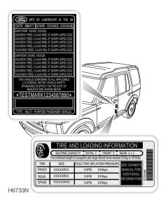
Two tire information labels are visible on the pillar behind the driver's door ( known as the  $\bf B$  pillar), giving information specific to the wheel and tire equipment fitted to the vehicle when it was built
