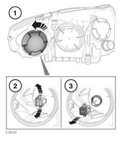
To gain more room for accessibility, follow the process for removing the headlamp unit. See 192. HEADLAMP REMOVAL.
