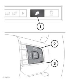
1. HDC on/off: HDC can be selected at any speed, but will only operate at speeds of less than 50 km/h (31 mph).
