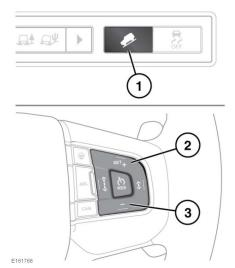
HDC on/off: HDC can be selected at any speed, but will only operate at speeds of less than 50 km/h (31 mph).
