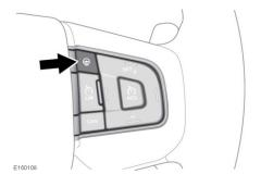
Press to switch on the steering wheel heating. Press again to turn off.
