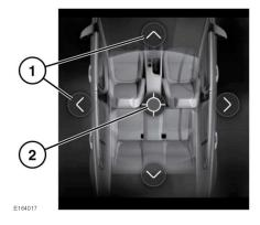
Touch the arrow soft keys (1) to move the sound focal point to the desired area of the vehicle. Alternatively, touch the sound focal point (2) and 'drag' it to the required position. To return to the default setting, touch the sound focal point (2).
