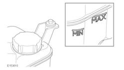
Make sure the coolant level remains between the **MIN** and **MAX** indicator marks on the side of the expansion tank.
