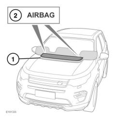
If your vehicle is fitted with a Pedestrain airbag, it is located beneath a panel in the bonnet (1).
