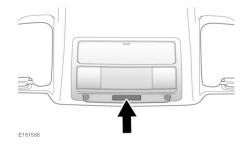
The warning lamp, mounted in the roof console, will display the operational status of the passenger front airbag, as shown in the following table.
