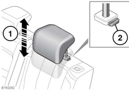
1. To raise, pull the head restraint upwards.
