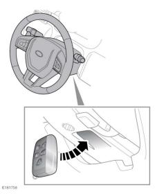
Position the Smart key flat against the underside of the steering column with the buttons facing downwards.
