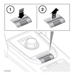
With the ignition turned on, press the brake pedal, then press down and release the EPB switch. This will release the EPB. 2. With the vehicle stationary, pull up and release the EPB switch. This will apply the EPB. The parking brake warning lamp will illuminate to indicate that the EPB is applied. See 53, PARKING BRAKE (RED).
