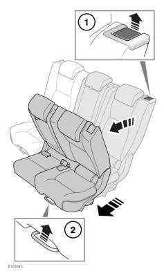
To tilt the seatback forwards: Pull the lever on the top of the seatback upwards (1) to release the locking mechanism, and then move the seatback forwards into the tilt position.
