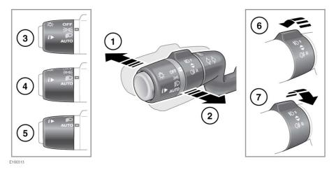
With the headlamps on, push the control away from the steering wheel to select high beam. The Instrument panel warning lamp will illuminate. See 57, HIGH BEAM (BLUE).
