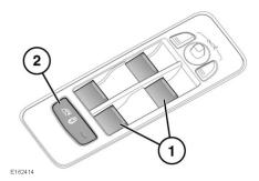
Window switches: Briefly pull a switch fully up and release; the window will continue to rise until fully closed. Briefly press a switch fully down and release; the window will continue to lower until fully open. Pressing or pulling a switch again will stop window movement.
