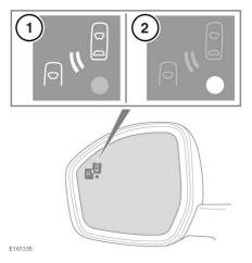
If an object is identified by the BSM system as being an overtaking vehicle/object, an amber warning icon (1) illuminates in the relevant exterior mirror, to alert the driver that there is a potential hazard in the vehicle's blind spot and therefore, that a lane change might be dangerous.
