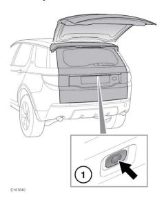
1. Press to release the tailgate and then lift the tailgate to open.
