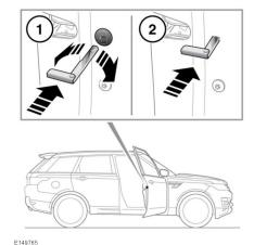
In the event of the battery discharging or a fault with the keyless locking system, the doors must be locked manually.
