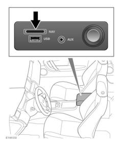
The Navigation SD card reader is located in the front centre cubby box. Make sure the SD card is located correctly in the card reader before operating the Navigation system.
