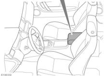
The Navigation SD card reader is located in the front centre cubby box. Make sure the SD card is located correctly in the card reader before operating the Navigation system.
