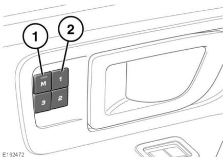
1. On the driver's door, press the memory store button (**M**) to activate the memory function. The switch indicator will illuminate.
