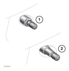
Wheels fitted with a TPMS can be visually identified by the external metal lock nut and valve (1). All Land Rover non-TPMS wheels have a rubber valve fitted (2).
