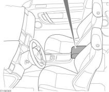
Connect the device into the appropriate socket:
