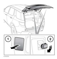
Replacing a reversing lamp bulb:
