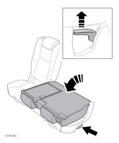
To fold a second row seatback: Lift the lever on the side of the seat and pull the seatback forwards until it locks into the lowered position.
