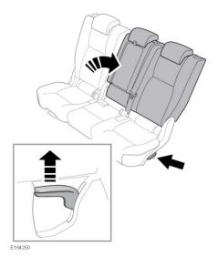
To recline the second row seatback: Lift the lever on the side of the seat and push the seatback into the recline position.
