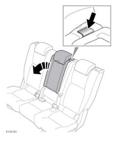
To fold the centre of the seatback: Press the release button on the top of the seatback, then fold the centre of the seatback forwards into the lowered position.
