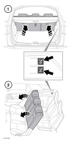
The second row seatbacks can be folded from inside the loadspace (1), or by the passengers occupying the third row seats (2):
