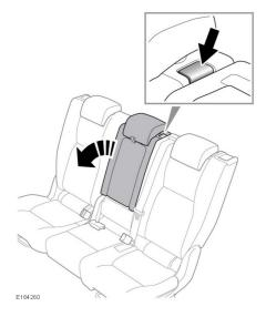
To fold the centre of the seatback: Press the release button on the top of the seatback, then fold the centre of the seatback forwards into the lowered position.
