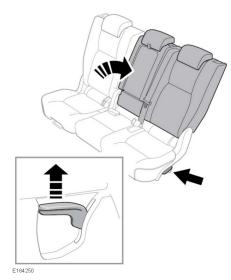
To recline the second row seatback: Lift the lever on the side of the seat and push the seatback into the recline position.
