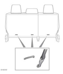
Your vehicle is equipped with anchorage points on the back of the second row seat frames. These should be used to attach straps from child seats or restraint systems.
