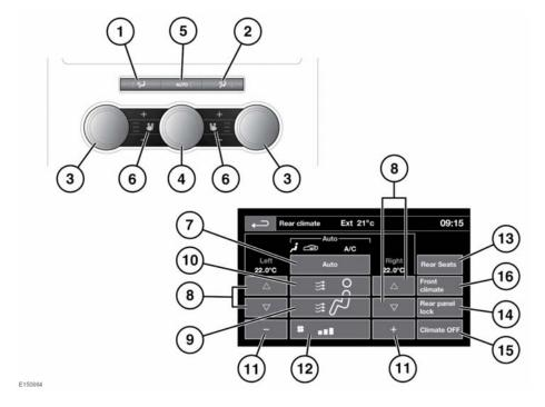
There are two types of Rear climate control: 3 Zone and 4 Zone. All of the 3 Zone controls will affect the whole of the rear passenger compartment. 4 Zone allows independent control of each side.
