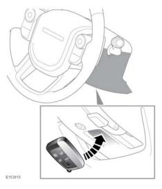
Position the Smart key against the underside of the steering column with the buttons facing downwards.
