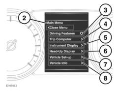
A number of vehicle features and display settings may be configured via the Instrument panel menu.
