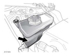
The fluid level should be maintained between the **MIN** and **MAX** marks.
