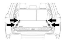
2. If adjustable lashing eyes are fitted, first turn the locking button counter-clockwise to unlock. Press the button and slide to the required position in the luggage rail. Release the button to latch into position. Move the lashing eye slightly, until you hear a click. The lashing eye is now secured. Turn the button clockwise to lock.
