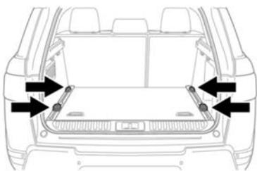
2. If adjustable lashing eyes are fitted, first turn the locking button counter-clockwise to unlock. Press the button and slide to the required position in the luggage rail. Release the button to latch into position. Move the lashing eye slightly, until you hear a click. The lashing eye is now secured. Turn the button clockwise to lock.
