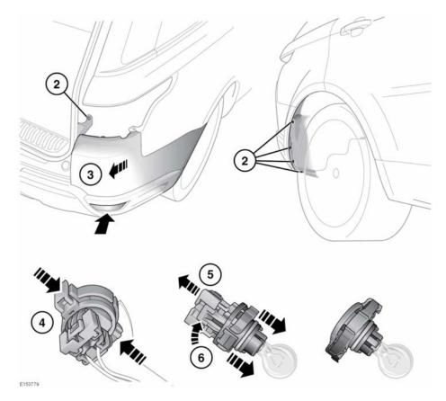
Access to a rear fog lamp housing is from above and behind the rear bumper. The bulb holder is a black plastic unit that incorporates the bulb. Set the Air suspension to the Off-road height position, for increased access to the bumper fixings. See **120**, **OFF-ROAD HEIGHT**.
