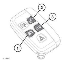
To raise the vehicle, press and hold button (1) and button (2) together.
