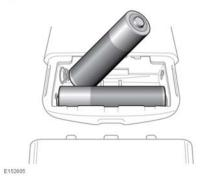
Low battery power is indicated by the remote control power button flashing 3 times when pressed. To renew the batteries:
