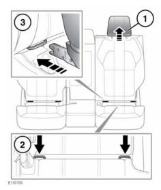
Both of the outer seat positions on the rear, second row seat are equipped to accept ISOFIX restraints.
