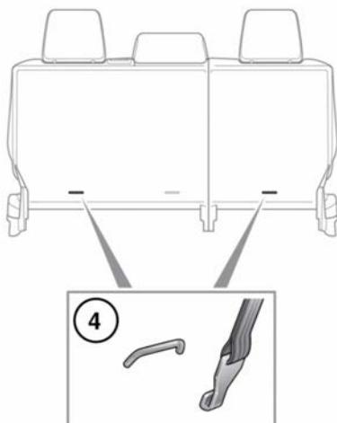
**Note:** Always make sure if an upper tether is provided, it is fitted and tightened correctly.
