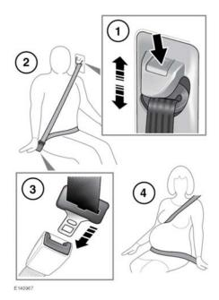
1. Seat belt height adjustment: Press to release the catch.
