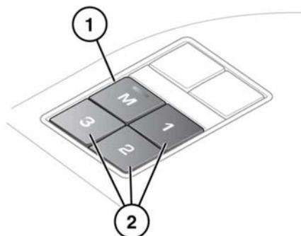
1. Press the memory (**M**) button to activate the memory function.
