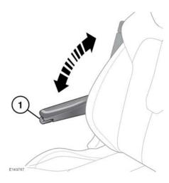
Use the adjuster wheel (1) to set the required height. The folding armrest may be stowed by moving to the vertical position.
