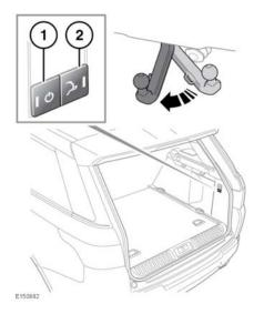
The Powered tow bar is hidden in its stowed position behind the bumper. It can be deployed using the buttons located on the right side of the loadspace.
