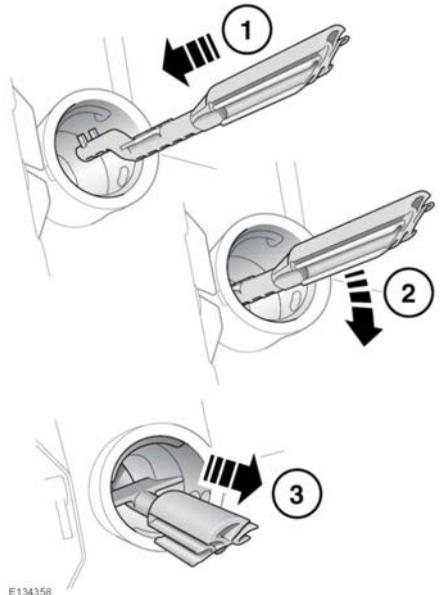
**Reset the Misfuelling protection device as follows:**
