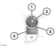
SET+: Press to set the speed or to increase the set speed. The Cruise control indicator illuminates to confirm that Cruise control is operational (see 54, CRUISE CONTROL (GREEN)).
