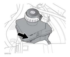
The driver's side cover must be removed to check the brake fluid level. See 221, UNDER BONNET COVERS - REMOVAL.
