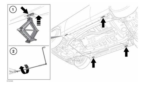
Before raising the vehicle, use the wheel nut brace to slacken the wheel nuts of the wheel to be replaced, by half a turn counter-clockwise.
