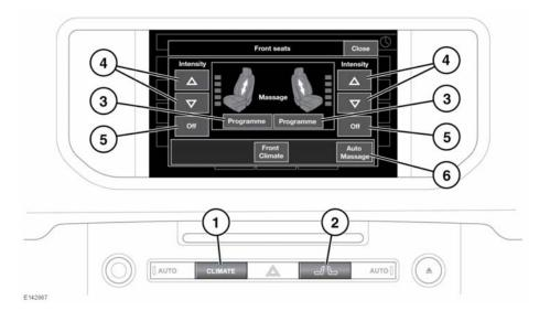
**Note:** Seat massage may not operate when the vehicle's interior temperature is below 0°C, or above 50°C (32°F or 122°F respectively).
