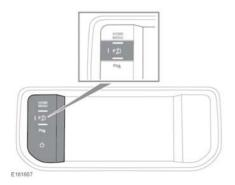
A short press of the Park assist button will turn the system on. When Park assist is switched on, the button LED will illuminate.
