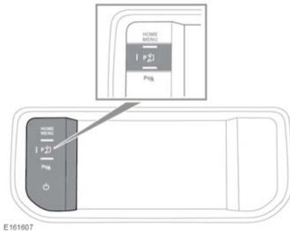
A short press of the Park assist button will turn the system on. When Park assist is switched on, the button LED will illuminate.
