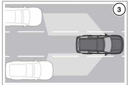
The Blind Spot Monitor (BSM) system monitors an area adjacent to your vehicle, that is not easily visible to the driver. The system is designed to identify any road user overtaking your vehicle (3) that is within this blind spot, while disregarding other objects which may be stationary or travelling in the opposite direction.
