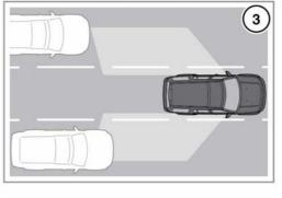
The Blind Spot Monitor (BSM) system monitors an area adjacent to your vehicle, that is not easily visible to the driver. The system is designed to identify any road user overtaking your vehicle (**3**) that is within this blind spot, while disregarding other objects which may be stationary or travelling in the opposite direction. *Note:* Refer to the warnings, cautions and notes at the beginning of this section for system limitations.
