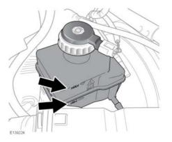
The driver's side cover must be removed to check the brake fluid level. See 235, UNDER BONNET COVERS - REMOVAL.
