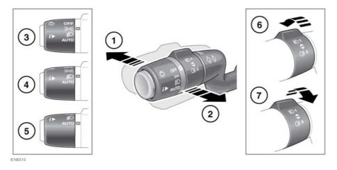
With the headlamps on, push the control away from the steering wheel to select high beam. The warning lamp will illuminate. See 53, HIGH BEAM (BLUE).
